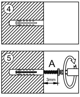
Make sure that the end of the wall plug is flush with the surface. Tighten the screw in the hole marked (A), leaving 3 mm space between wall and schrew head.
